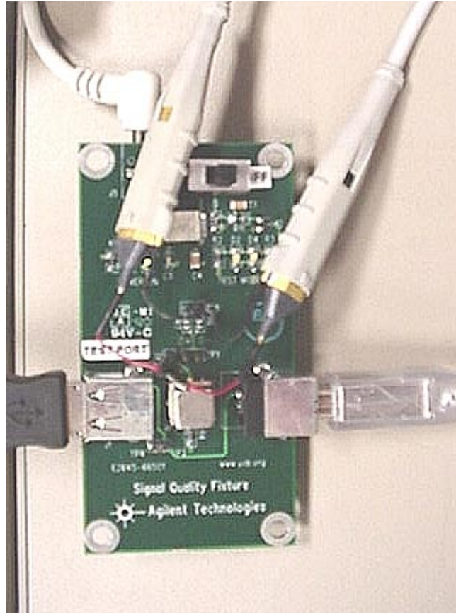
Figure 23. Probe Connection for CHIRP Testing
