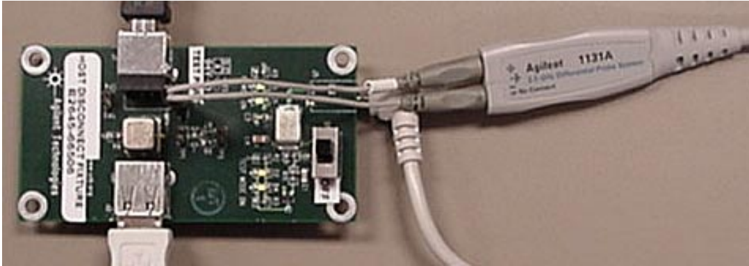
Figure 18: Differential Probe Connection on Host Disconnect Test Fixture
