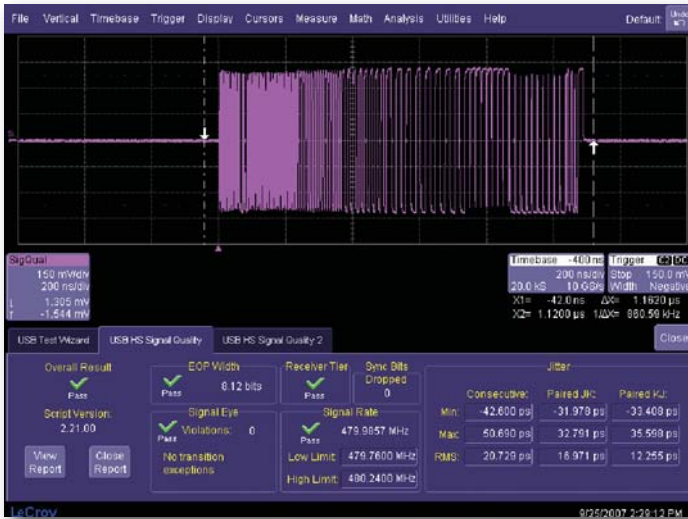
High-speed upstream signal quality test result.
