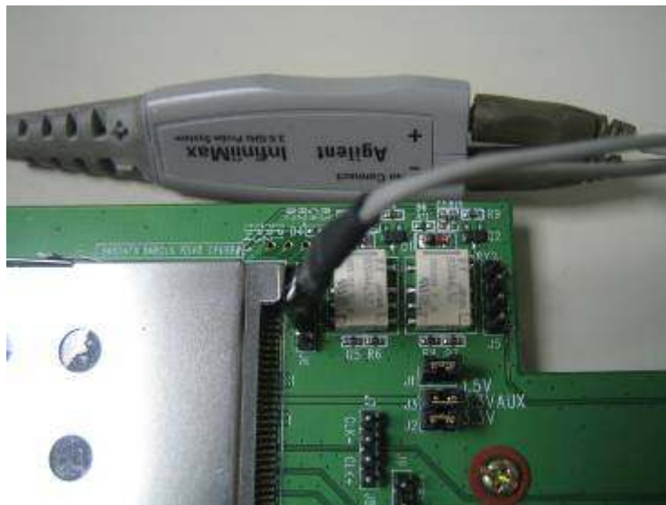
Figure 3-4: Differential Probe Connection
