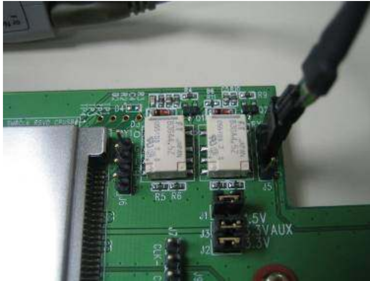
Figure 4-4: Differential Probe Connection
