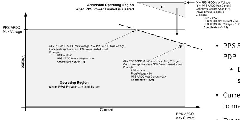
PPS Source limits its output power to the PDP
