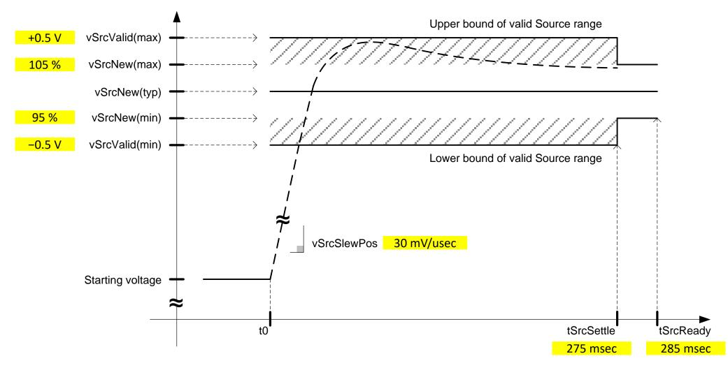
• The voltage limits to do not apply to vSafe0V and vSafe5V
