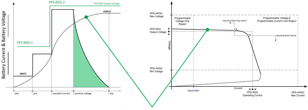
DECREASING charging current & HIGH battery voltage PPS in Constant Voltage mode Operating Mode Flag is cleared
