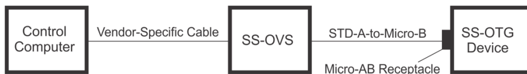
Figure 8-20 Alternate Test Setup for SSPC-OTG Device
