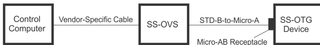
Figure 8-13 Alternate Test Setup for SS-OTG A-Device
