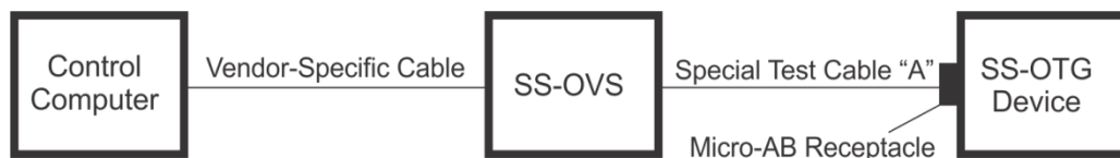
Figure 8-15 Alternate Test Setup for SS-OTG A-Device
