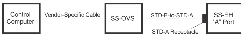
Figure 8-6 Alternate Test Setup for SS-EH (SS-EH using STD-A Receptacle)
