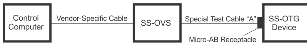
Figure 8-13 Alternate Test Setup for SS-OTG A-Device
