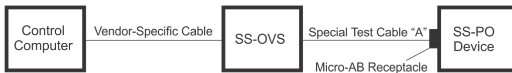
Figure 8-17 Alternate Test Setup for SS-PO Device (SS-PO using Micro-AB Receptacle)
