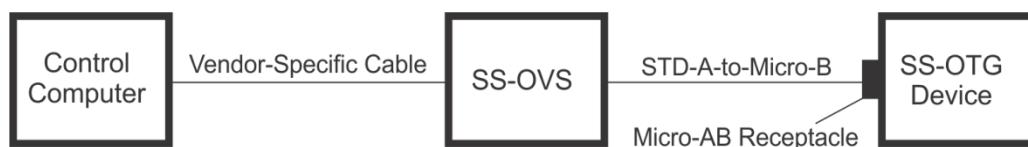
Figure 8-15 Alternate Test Setup for SS-OTG A-Device
