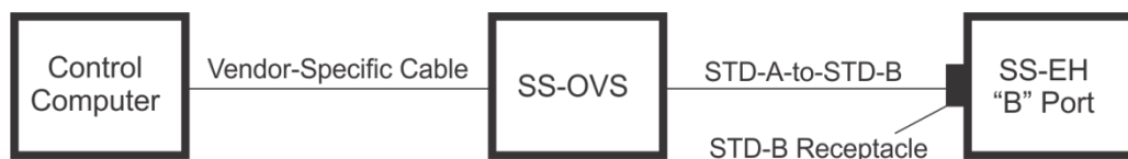
Figure 8-9 Alternate Test Setup for SS-EH (B-Port using STD-B Receptacle)
