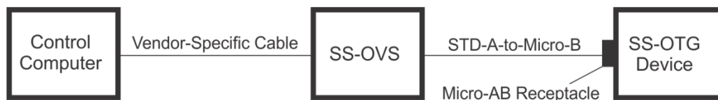
Figure 8-11 Alternate Test Setup for SS-OTG Device (Common Tests)
