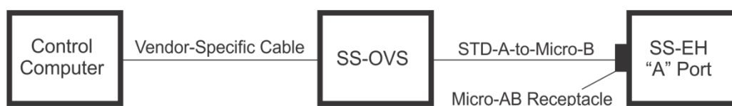
Figure 8-6 Alternate Test Setup for SS-EH (SS-EH using STD-A Receptacle)
