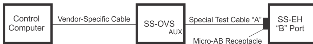
Figure 8-7 Test Setup for SS-EH B-Port (B-Port using Micro-AB Receptacle)
