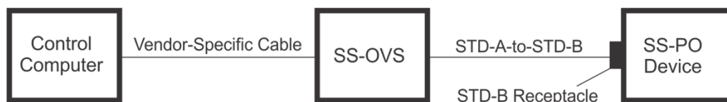
Figure 8-18 Alternate Test Setup for SS-PO Device (SS-PO using STD-B Receptacle)
