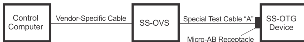
Figure 8-11 Alternate Test Setup for SS-OTG Device (Common Tests)
