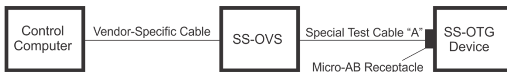
Figure 8-20 Alternate Test Setup for SSPC-OTG Device
