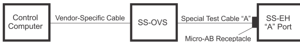
Figure 8-4 Alternate Test Setup for SS-EH (SS-EH using Micro-AB Receptacle)
