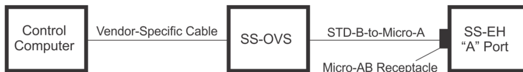
Figure 8-5 Special Setup for SS-OVS A-Port Connected via Micro-B to SS-EH A-Port
