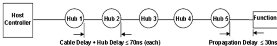
Figure 7-41. Worst-case End-to-end Signal Delay Model for Low-/full-speed
