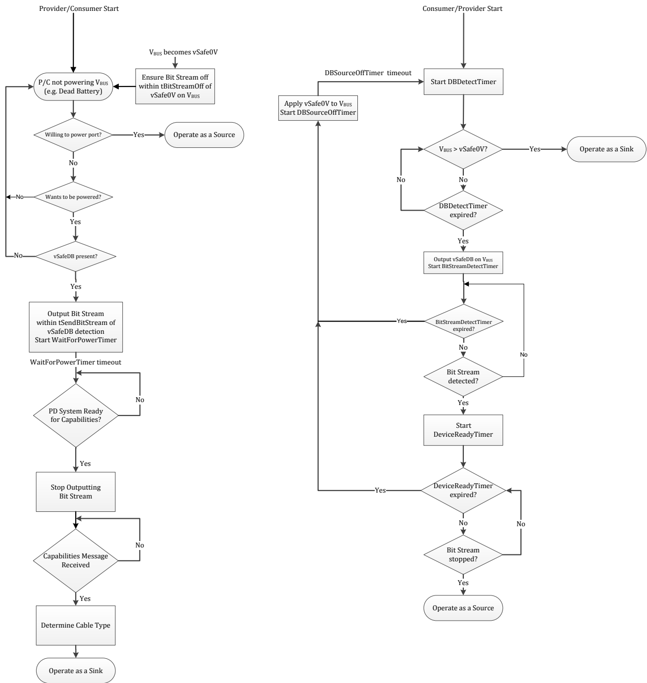
Figure 4-1 USB Type-A to USB Type-B Dead Battery / Unpowered Port Detection Flow
