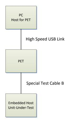
Figure 6-2 Setup No 2 – Embedded Host
