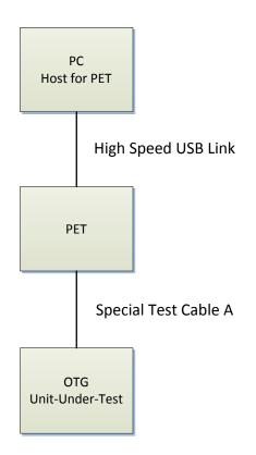
Figure 6-1 Setup No 1 – OTG Device
