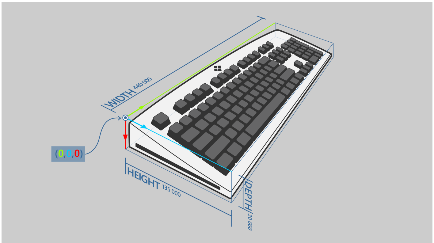
Figure 25.2: Keyboard with labeled dimensions and origin. Lamps exist beneath every key, the branding at the top/middle, and accent lighting along the left and right sides. Example sizes given for each dimension (in \mu\text{m} ).
